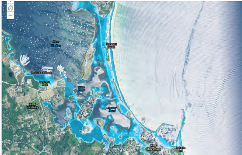
25-year storm event (4% chance of occurring in any given year) with 1 foot of Sea Level Rise.
